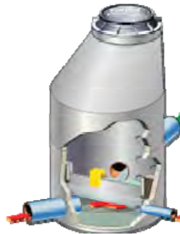
Figure 5-4: StormGate™ proprietary flow splitter structure. Source: Contech Construction Products Inc. The use of this illustration is for general information only and is not an endorsement of this or any other proprietary device.
