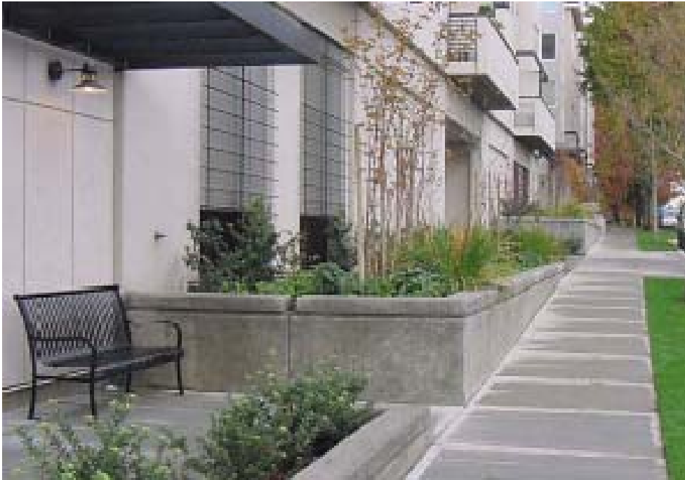
Figure 6-22: Flow-through planters. Source: City of Portland
