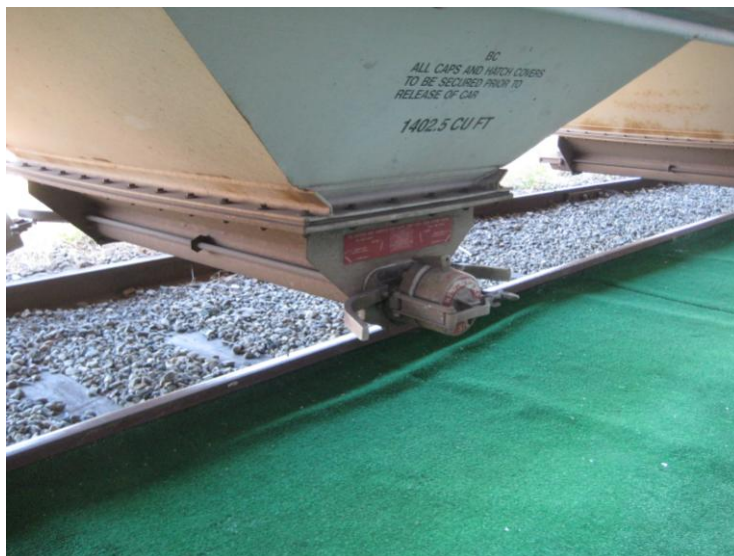
Photo 1d & 1e. Proper seal and containment systems for pellet transfer, 2011, ePoly Star.
