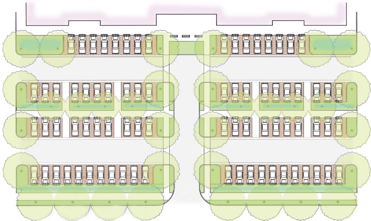
Figure 2-19: A redesigned parking lot using 15 foot long parking stalls and 22 foot wide vehicle travel aisles yields significant amounts of landscape space that can be used for stormwater management. This example also has improved pedestrian circulation within the parking lot.
