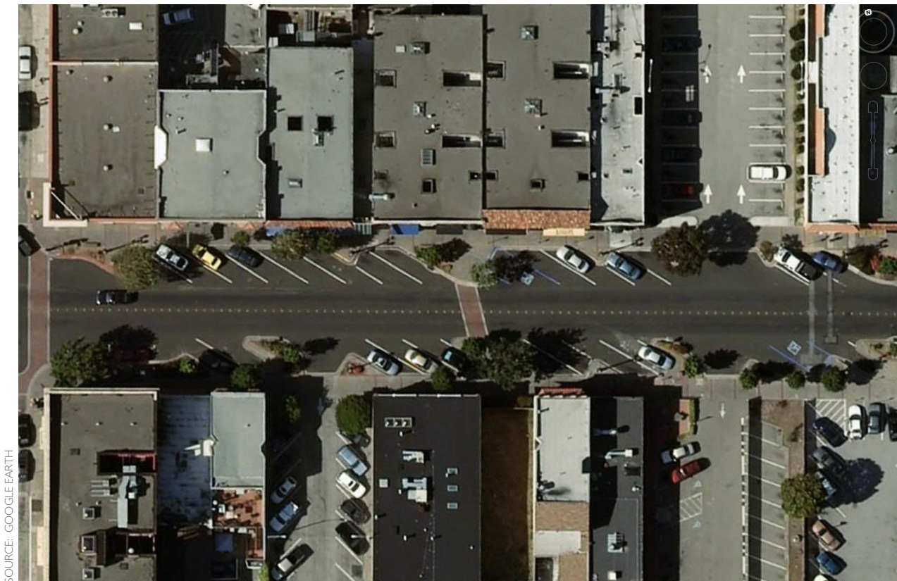
Figure 2-13: An aerial view of a commercial main street using 30 degree angled on-street parking. Notice how much space is wasted at the back end of each oversized parking stall. Also notice the narrow the sidewalk zone.
