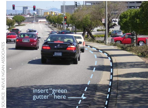
Figure 2-91: Green gutters can often be installed parallel to an excessively wide travel lane. Dashed lines show where a green gutter could be added.
