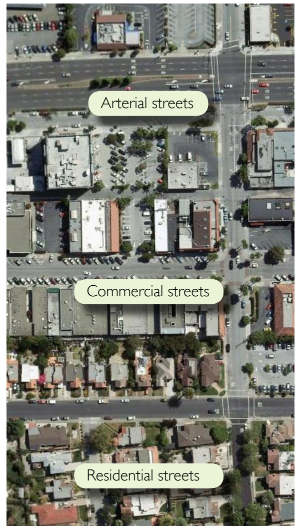
Figure 3-1: Residential, commercial, and arterial street types can be found in close proximity to each other in San Mateo County. However, the design solutions for each can vary considerably in complexity.
