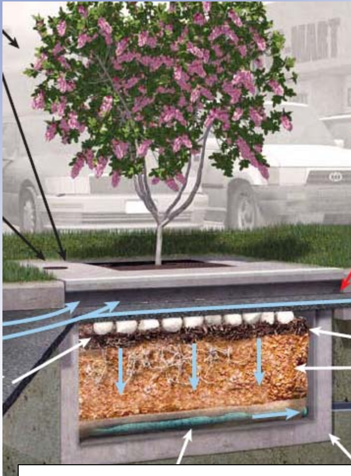
Example of a Manufactured Tree Well Filter
