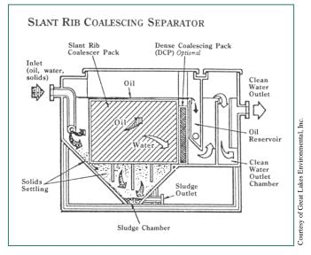
A CPI separator can be very effective at removing oil but requires upstream sediment control and can be costly to maintain.
