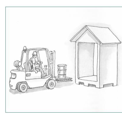
If the materials frequently leak during transfer, or the materials generally cause a wet environment when using or storing them, the area may need to be connected to the sanitary sewer (permitted by your wastewater authority), and should be covered and bermed to minimize contact with storm water.
