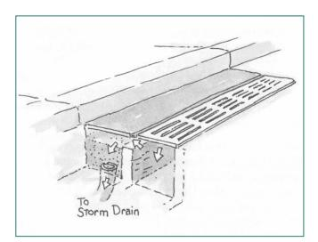
A sand filter inlet can remove some pollutants before they enter the storm drain.
