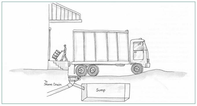
A dead-end sump provides secure spill control, but any accumulated liquids need to be pumped out, tested, and properly disposed. Use berms or slopes to prevent run-on so storm water is not added to waste in the sump.
