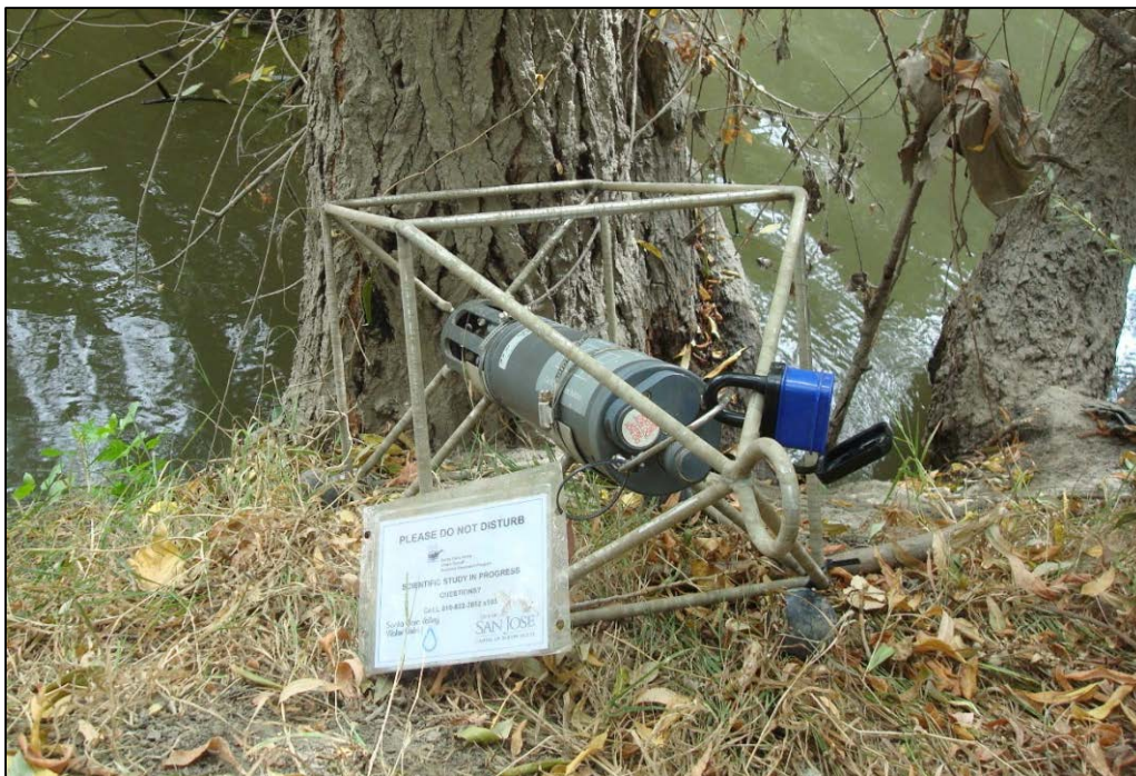
Figure 7. Photograph of sonde within metal cage, showing how probes would be elevated approximately six inches off the stream bed.
