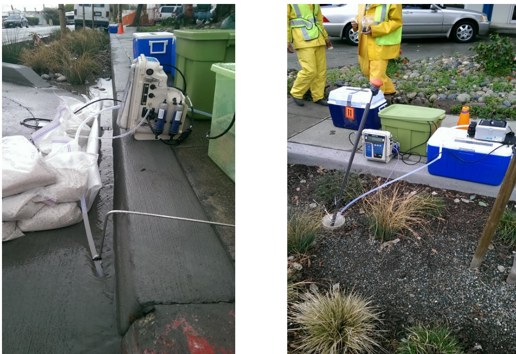
Figure 2. Influent (left) and effluent (right) sampling locations at site PUL-7 on Bransten Road, City of San Carlos.
