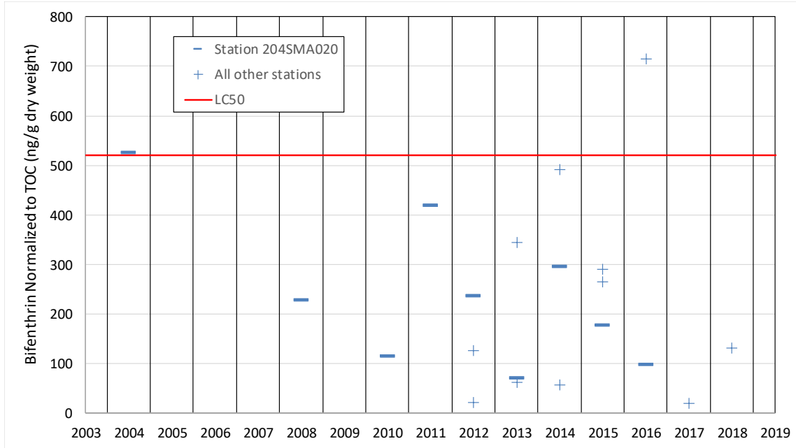
Figure 4-2. Bifenthrin concentrations in bedded sediment collected from San Mateo County urban creeks from 2004 to 2018. The red line is the adverse effects concentration (i.e., LC50) for Hyalella azteca (Amweg et al. 2005). Only samples with concentrations above the detection limit are included
