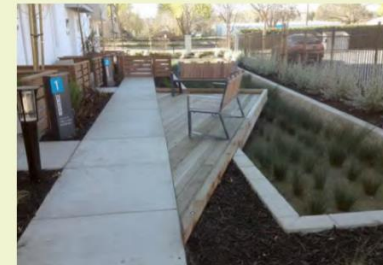
▲ EXAMPLE: An example high-density residential rain garden captures roof runoff and features a boardwalk overlook and seating area.
