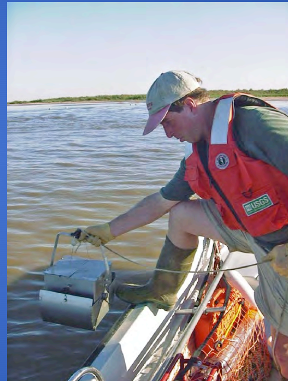
Sampling sediments for pyrethroids
