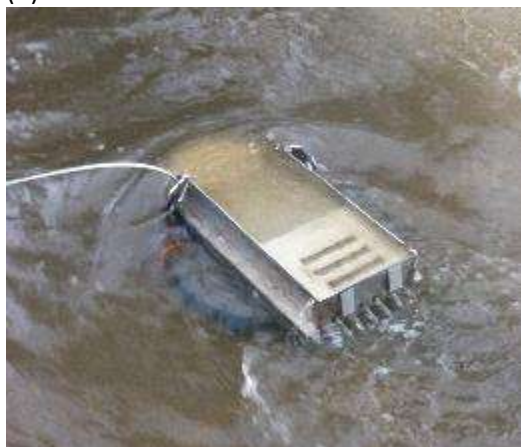
Figure 2. Sampling equipment used in the field. (a) Painters pole, Teflon tubing and an ISCO used as a slave pump; alternatively a Teflon bottle is attached to the end of a painters pole (DH84) and used for sample water collection as opposed to using an ISCO as a pump (b) Hamlin suspended sediment sampler; and (c) the Walling tube suspended sediment sampler.
