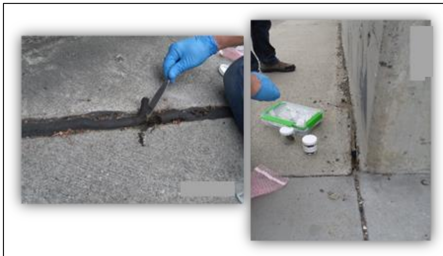
Figure 3.5 Examples of structures that were sampled and caulk materials that were included in Composite A, which had Very High PCBs ( \geq 1,000 ppm).
