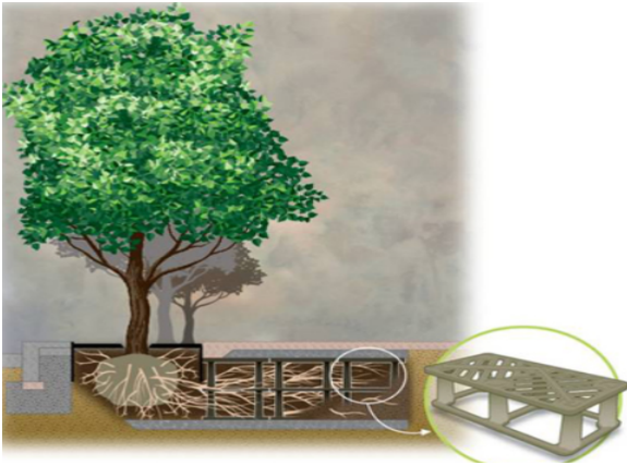
Figure 1-5 Stormwater tree well filter example
