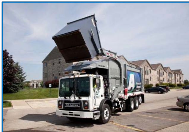
Figure 26. FEL (Front-End-Loading) vehicles tip bins into a hopper on top of the vehicle with poor wind protection
