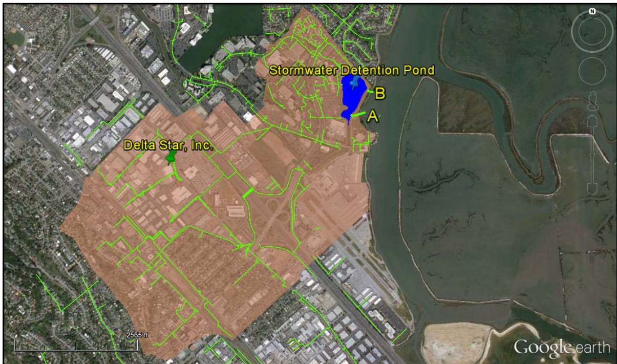
Figure 4.1. Drainage catchment and storm drain lines for the Redwood Shores Ecological Reserve Stormwater Detention Basin in Redwood City (shown in blue). Point A is the pump station discharge pipe location. Point B is the gravity fed discharge pipe location. Both discharge pipes empty to the Steinberger Slough.
