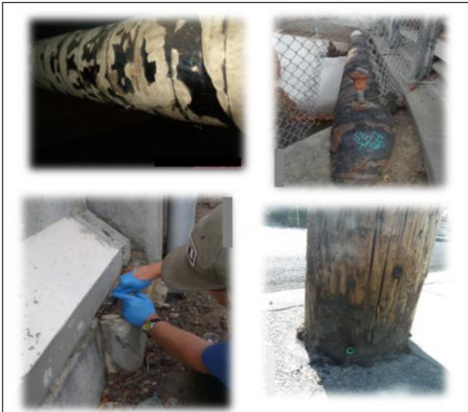
Figure 3.4 Examples of structures that were sampled and sealant materials that were included in the composites that had Moderate PCBs ( \geq 1 ppm and < 50 ppm). Not all structures/samples in the Moderate PCBs category are pictured here.
