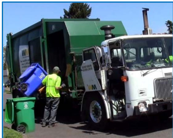
Figure 25. Side-loading vehicle tipping carts into hopper with good wind protection
