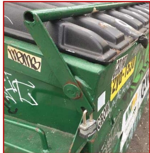
Figure 30. Locking lid on Front End Load (FEL) container.
