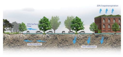
The use of green infrastructure allows for a balanced approach to urban development, as it accommodates existing infrastructure while minimizing the detrimental effects on the natural system. The use of green infrastructure such as permeable surfaces, bioswales, and green roofs allows for greater
