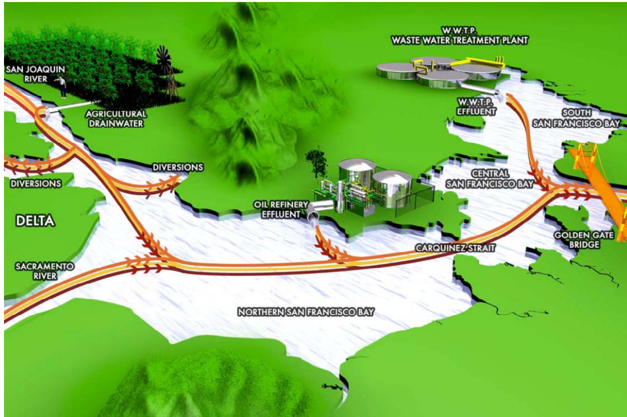
Figure 4-1. Generalized conceptual model of selenium sources and pathways in San Francisco Bay (Abu-Saba and Ogle 2005).
