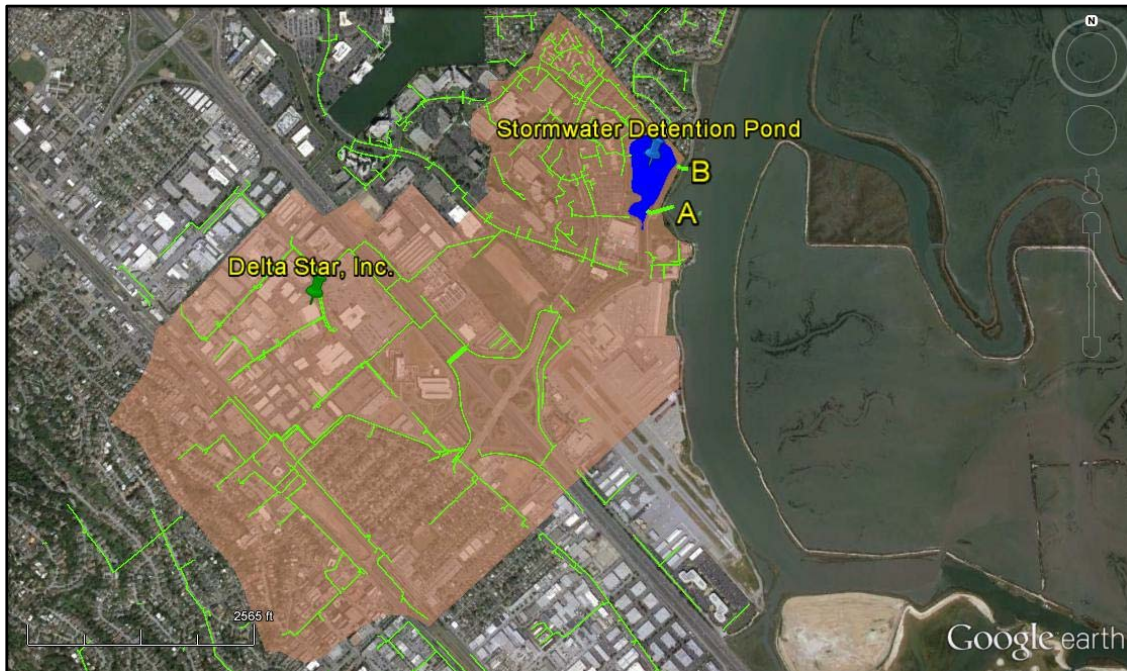
Figure 4.1. Drainage catchment and storm drain lines for the Redwood Shores Ecological Reserve Stormwater Detention Basin in Redwood City (shown in blue). Point A is the pump station discharge pipe location. Point B is the gravity fed discharge pipe location. Both discharge pipes empty to the Steinberger Slough.
