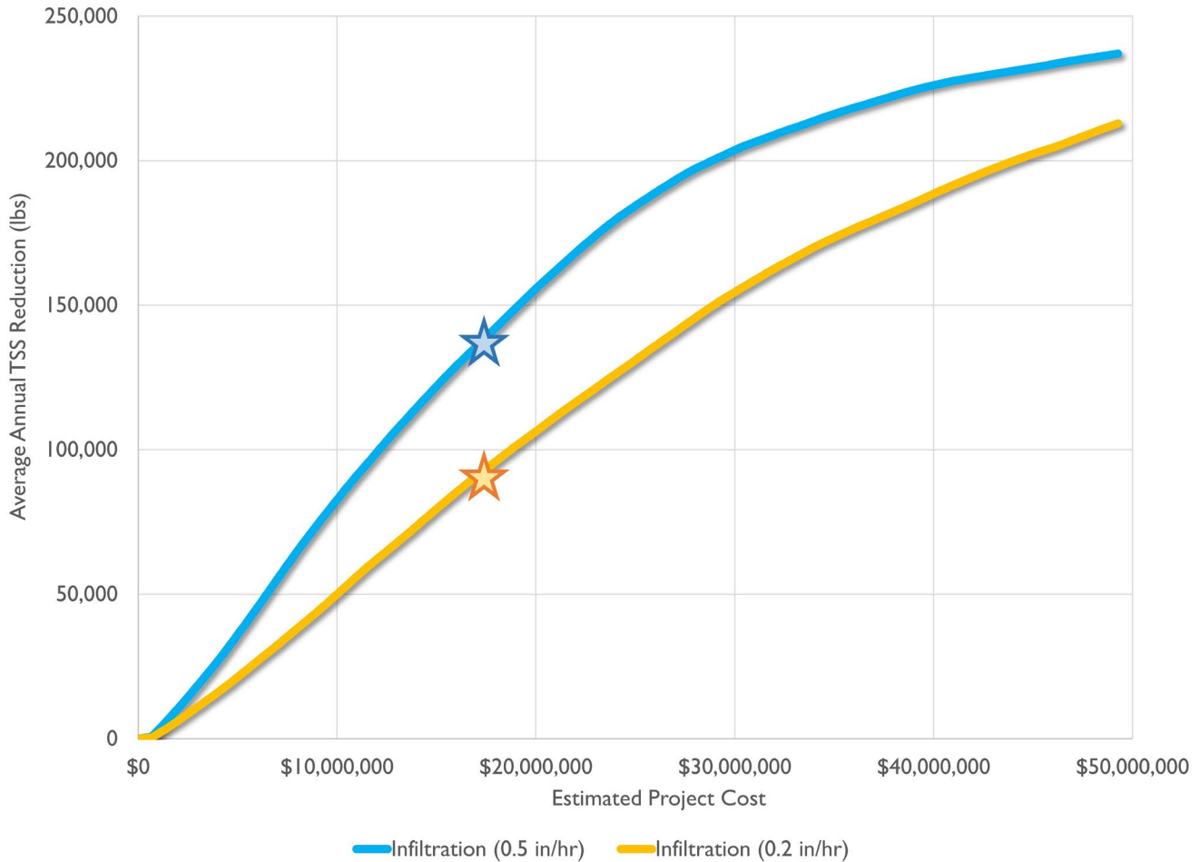
Figure 2-7. Estimated project cost vs pollutant reduction for a BMP with a 70 cfs diversion rate at the project site.
