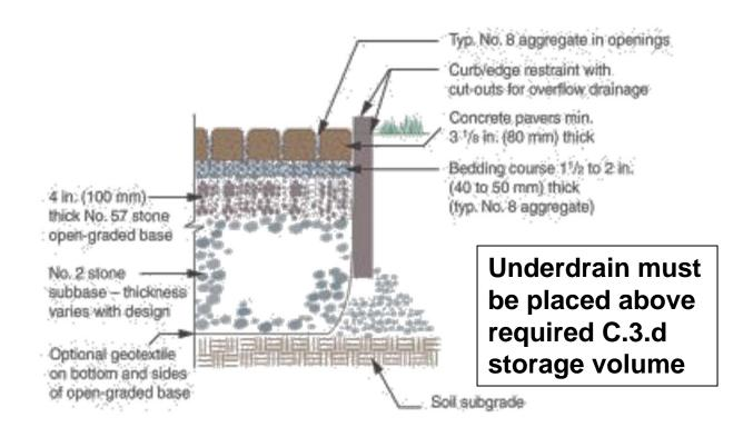
Permeable interlocking concrete paver section (Source: ICPI)
