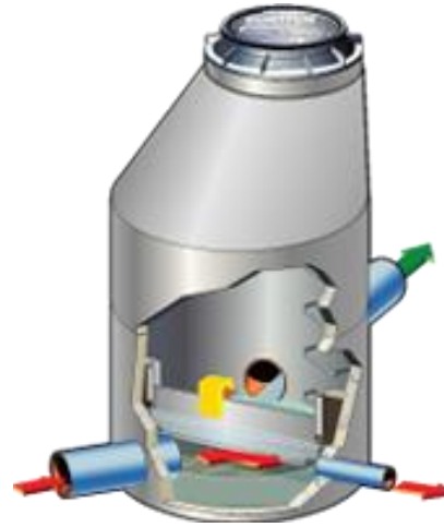
Figure 5-2: StormGate™ proprietary flow splitter structure. (Credit: Contech Construction Products Inc). The use of this illustration is for general information only and is not an endorsement of this or any other proprietary device.
