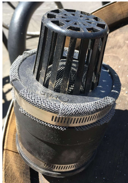
Figure 3: Inlet filter made of atrium grate, screening and rubber fernco
